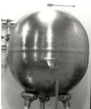
Figure 5-2: all titanium construction (typically hot forged, solution treated, quenched and aged 6Al-4V alloy, which if possible, is weld stress relieved after assembly.) This particular tank is PSI 80375, four of which were used in Judith 0702's second stage. It is currently used as the main fuel tank for the Iridium phone satellite, where it is launched filled with hydrazine. For Mars Challenger , it was launched empty from Earth and filled with propellant after arriving on Mars.
