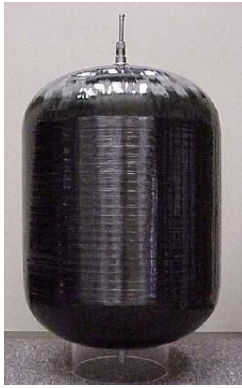
Figure 5-3: full carbon fibre reinforced composite overwrapped titanium liner, a method currently exclusive to pressurant tanks. The welded titanium liner provides the hermetic seal, while composite overwrap bears the pressure stresses. This example is PSI's 80446, which is used as the main lander helium tanks for Judith . The lander's cryocoolers, and booster's smaller bottles are charged from these tanks. The second stage of Judith 0710 uses tanks of similar appearance to this one, but with the operating pressure and actual size somewhat larger than the titanium tank shown in Figure 5-2. These second stage tanks carry the hydrogen, and as a result, require an aluminum liner since titanium is severely embrittled in the presence of hydrogen.
