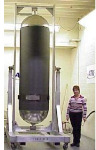
Figure 5-3: full carbon fibre reinforced composite overwrapped titanium liner, a method currently exclusive to pressurant tanks. The welded titanium liner provides the hermetic seal, while composite overwrap bears the pressure stresses. This example is PSI's 80446, which is used as the main lander helium tanks for Judith . The lander's cryocoolers, and booster's smaller bottles are charged from these tanks. The second stage of Judith 0710 uses tanks of similar appearance to this one, but with the operating pressure and actual size somewhat larger than the titanium tank shown in Figure 5-2. These second stage tanks carry the hydrogen, and as a result, require an aluminum liner since titanium is severely embrittled in the presence of hydrogen.
